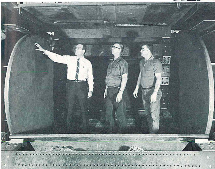
Hardy Stebbins, Sales Manager of Standard Blast Equipment, Ray Lidgard, and Ray Spice are examining the constructional features of barrel head wear plates on one of two 100 cu. ft. Super Tumbblasts being built for Boston Naval Shipyard and Norfolk Naval Shipyard, Portsmouth, Virginia, for the cleaning of anchor chain.
